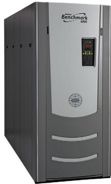
The BMK6000 has an operating efficiency of 94.5 percent to reduce operating expenses and yield the highest possible seasonal fuel savings. The BMK6000 measures only 79 H x 34 W x 109 D (inches). The BMK6000's 439 stainless steel construction helps the boiler achieve high efficiency, improve longevity and create greater heat exchanger cycling resistance.
